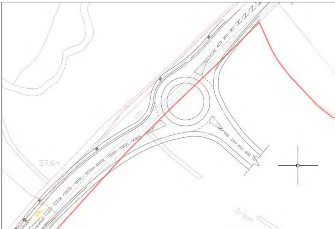
Figure 5.1: Existing UKPN Cables (in red) that may require protecting or diverting
